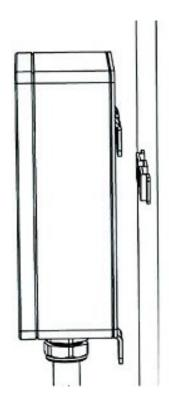
5. **Optional:** Use a wall screw (x1) to secure the bottom of the enclosure bracket to the wall.
